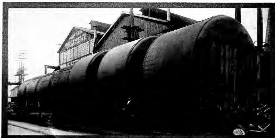
Seven Scotch marine boilers awaiting shipment from the plant of the Willamette Iron and Steel Works, Portland, Oregon.
